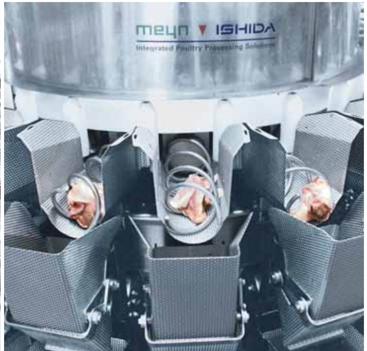
Spiralförderer transportieren das Fleisch kraftvoll und schonend in die Schalen. Spiral conveyors transport the meat forcefully and gently into trays.
