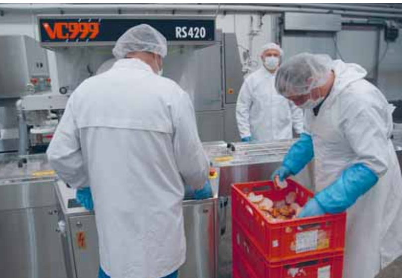
An der VC999 RS420 verpackt Nordfrost vor allem SB-Produkte. / On the VC999 RS420 Nordfrost mainly seals self-service products.
