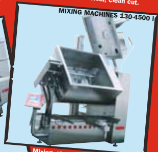
Mixing, standardizing or homogenizing large batches and massaging ham, equipped with Z-shaped mixing arms, mixing paddles and spirals.
