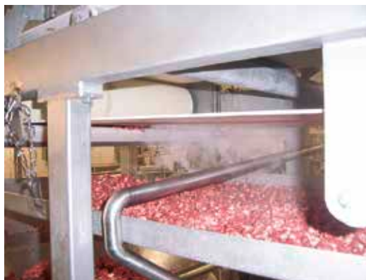
Abb. 2: Vernebelung an der Hackfleischlinie/ Fig. 2: Misting on the minced meat line.
